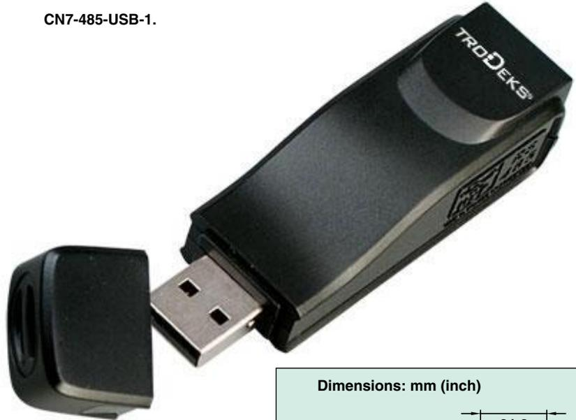
The CN7-485-USB-1 mini-node communication signal converter is a low cost device that converts half duplex RS485 serial communications signals into a signal that can be read by any computer with a USB port. The integral USB connector and RJ-45 connector reduces set up time by eliminating extra wiring. The CN-485-USB-1 is powered via the USB connection which eliminates the need for an external power source. The compact size is great for field installation, control panels, and lab testing.
