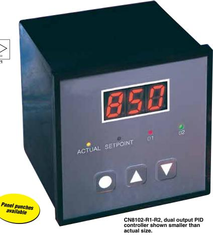
ovens and packaging machinery. As a high-limit device, these controllers have a normally energized SPST latching output relay which becomes de-energized whenever the process variable (PV) exceeds a selected setpoint value. Reset of the latching output relay is done by holding the parameter button for 3 seconds on the front panel of the controller, or by cycling power to the controller.
