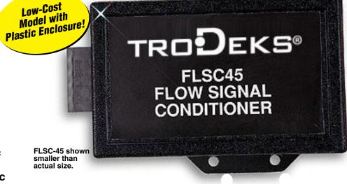
The FLSC-45 flow signal conditioner is a DC-powered, frequency-to-analog converter that interfaces directly to many of TRODEKS's paddlewheel sensors to provide a linear scaled 4 to 20 mA or 1 to 5 Vdc field-
