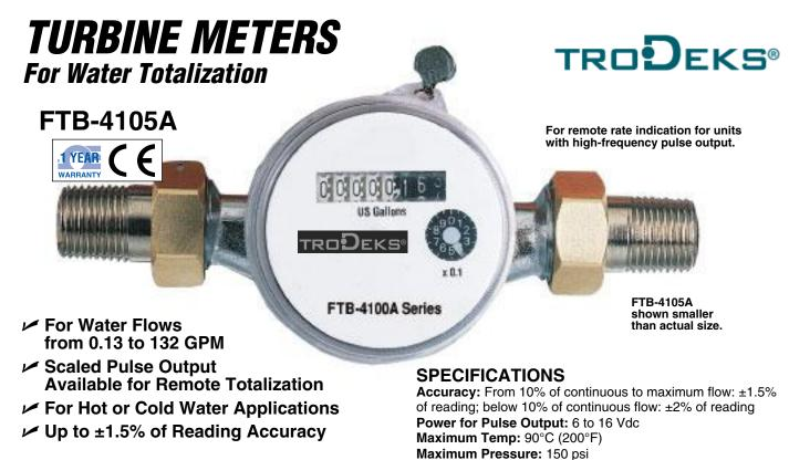
Designed for water billing applications, TRODEKS's FTB-4100A flowmeters are highly accurate and feature tamper-resistant, non-resettable totalizers. The large faces are easy to read.
