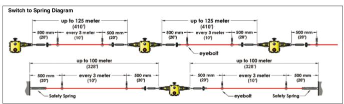
**Note:** It is important that the first 500 mm (19.68") is not used as part of the active protection coverage. If protection is required in this first 500 mm (19.68") then it is recommended to use switches fitted with a mushroom type E-Stop button. **TRODEKS** also recommends using a safety spring when a maximum of one corner pulley is used.
