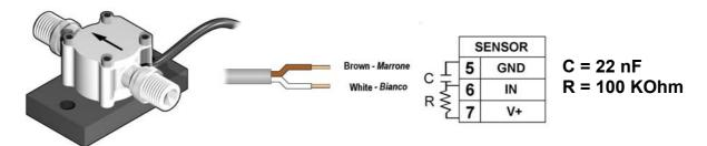
The capacitor C and the resistor R are already included if the sensor is bought together with the FlowX3 Battery Powered Monitor F9.20.XX.
