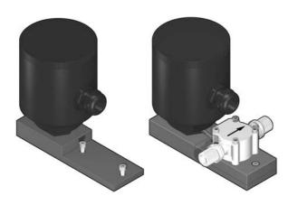
This Kit consists of an additional IP65 housing mounted aside the sensor via a PVC plate. It is a blind transmitter designed to convert the signal from the sensor into a 4...20 mA output for long distance transmission.
