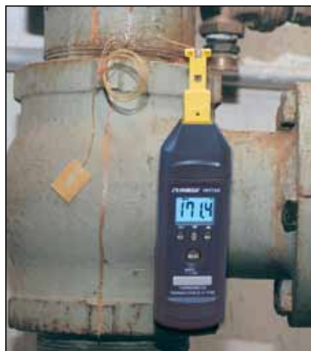
HH74K shown with optional SA1-K-SC, self-adhesive thermocouple.
