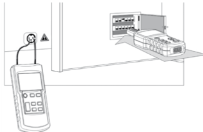
Identifying the fuse or circuit breaker associated with an AC outlet
