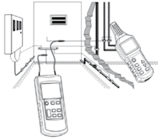
Locating a cold (left) or hot (right) metal water pipe
