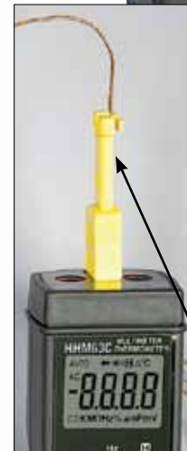
HHM63C/HHM63F Multimeter Thermometer 2500 count resolution W/microprocessor-based DMM DCV accuracy: 0.25% Resistance accuracy: 0.3% Backlit LCD display Frequency accuracy up to ± 0.05% Frequency resolution up to 0.001 Hz Type K input Temp. accuracy ± 2%
