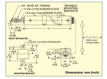
**Shaft:** 6 mm (0.236") diameter with ½-28 threaded-end adaptor
