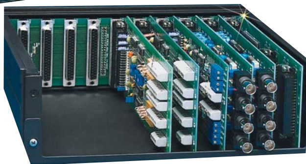
The OMB-DBK41, $879, provides slots for up to 10 analog expansion cards
