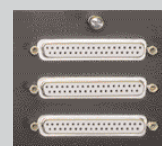
DB37-style termination panel (OMB-DBK608) features three standard 37-pin female connectors
