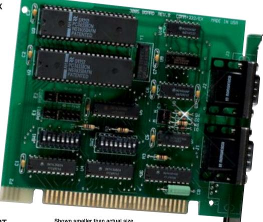
The OMG-COMM232-EX is a PC bus plug-in card based on the 16550 FIFO buffered UART, which is compatible with the standard 8250. This dual channel asynchronous serial communication card utilizes the RS-232 specification to provide RS-232 communication capabilities to your application. Selectable and sharable extended "AT" interrupts increase the OMG-COMM232-EX versatility. Signals are transmitted and
