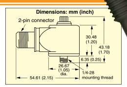
Mounting: ½-28 screw Output Connector: 2 pin, MIL-C-5015 style Connections: Pin A: Power/signal Pin B: Common
