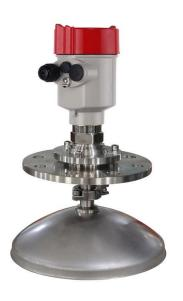
Application: Solid material, Strong dust, easy to crystallize, condensation occasion Measuring Range: 80 meters Process Connection: Thread, Universal Flange Process Temperature: -40°C~130°C (Standard type) -40°C~230°C (High temperature type) Process Pressure: -0.1 ~ 0.3 MPa Measurement Accuracy: ± 15mm Protection Grade: IP67 Frequency Range: 26GHz Display: LED, Programmable Supply: 2-wire (DC24V) / 4-wire (DC24V /AC220V) Signal Output: 4... 20mA / HART (2-wire / 4-wire ) RS485/ Modbus
