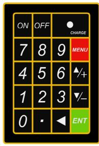
(2) Pressing  $\blacktriangle/+$  and  $\bigtriangledown/-$  keys. Each time of the  $\blacktriangle/+$  key pressing will proceed to the Lower - numbered menu window. For example, if the current window is on M12, the display will go to the number M11 window after pressing the  $\blacktriangle/+$  key.
