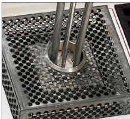
CL950 multi-well accepts up to 5 probes at one time and comes standard with \frac{1}{16} , \frac{1}{8} , \frac{3}{16} and two \frac{1}{4} " diameter holes.
