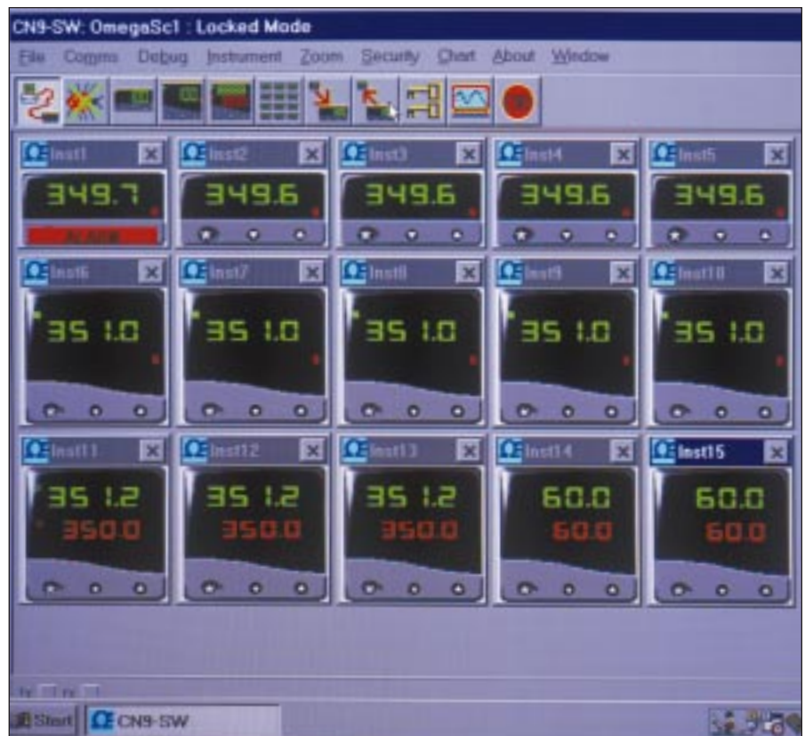
Screen displaying alarm condition on instrument 1. Software alarms provide a screen indication if the measured value falls below the low alarm and/or rises above the high alarm settings.
