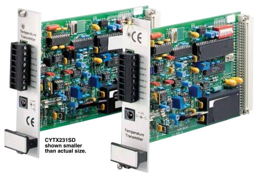
Electronic Accuracy: CYTX231SD, ±0.07 K at 4.2 K: CYTX231P ±0.15 K at 77 K
