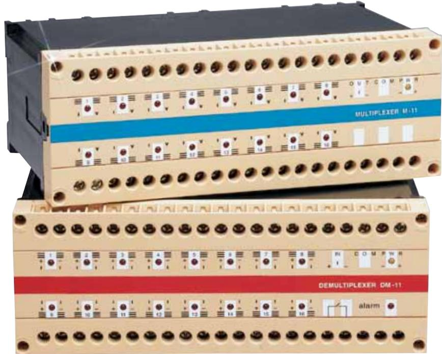
The DRA-MDM-11 is a mux/demux system which transfers analog information accurately via a single pair of wires. The multiplexer unit (DRA-M-11) accepts up to sixteen 4 to 20 mA process current inputs. The multiplexed inputs are transferred to the demultiplexer unit (DRA-DM-11) at a scan rate of up to 1000 channels/sec up to a distance of 2 kilometers (1.2 miles).
