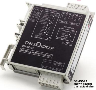
The DRI-DC-LA is a DIN rail mount, DC voltage or current input limit alarm with dual setpoints and two contact closure outputs. The field configurable input and alarm functions offer flexible setpoint capability. Input voltage spans from 10 mV to 200 V and input current spans from 1 mA to 100 mA can be field configured. Bipolar inputs are also accepted.
