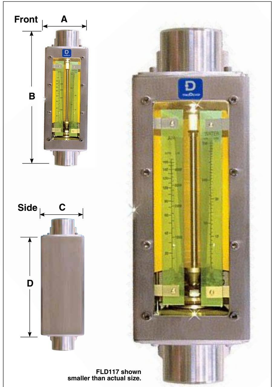
The FLD100 Series heavy-duty flow meters are fully enclosed in a brushed stainless steel case. Ideal for industrial applications with flow rates up to 116 GPM and 250 SCFM. Used with industrial water and air service. Meters are graduated for direct reading of water and air. Flow meters come standard with FNPT end fittings for easy in-line installation or ANSI 150 flanges (-FL)
