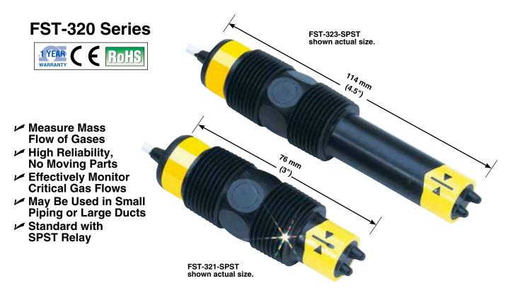
TRODEX's FST-320 Series thermal dispersion flow switches, especially designed for use with gases, sense changes in the heat transfer characteristics of the gases. Flow velocities from 1 to 90 fps are effectively monitored. The flow switch incorporates a standard SPST Relay switch output for control flexibility. TRODEX® controllers can easily be interfaced to perform a variety of control functions. The FST-320 family of sensors can be easily installed in line sizes ranging from ¾ to 12".
