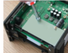
Figure 1 Unscrew the two nuts
