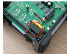
Figure 3 The black rectangular component is fuse
