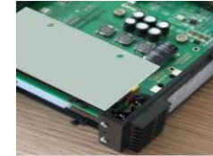
Figure 2 Remove the high voltage protection board
