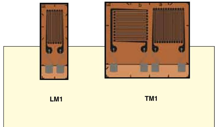
M Series strain gages have been specially developed for high resistance to alternating loads at increased strain levels and high temperatures up to 300°C (572°F). They are foil strain gages with measuring grids made of a special nickel-chromium alloy. TRODEX/HBM offer this special strain gage with various geometries, measuring grid lengths and temperature response matching.
