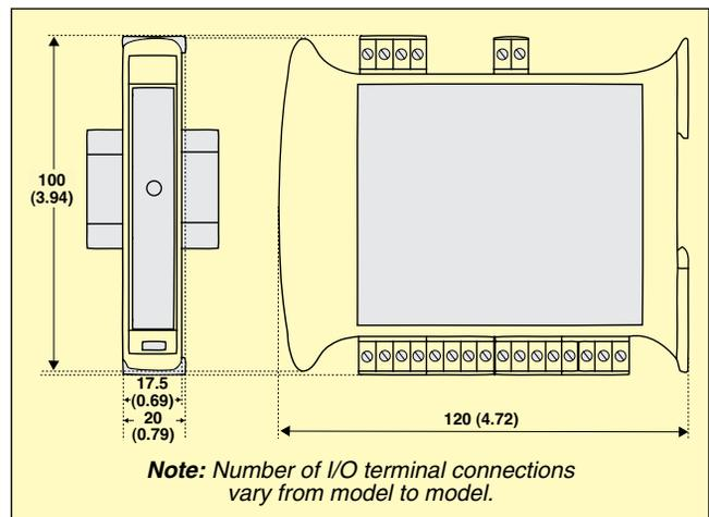
**Dimensions:** 17.5 W x 100 H x 120 mm D (0.69 x 3.94 x 4.72")**Weight:** 150 g (6 oz); 210 g (8.4 oz) HE359DIQ512 only**Communications:** MODBUS®/RTU (binary) RS485 half duplex**Default Communications Parameters:**
