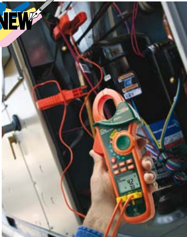
Dual Type K inputs for taking differential temperature readings needed for superheat measurements.
