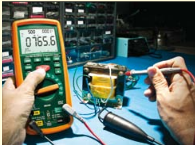
Measure the insulation resistance of transformer windings
