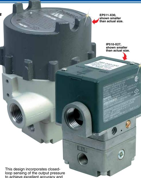
to achieve excellent accuracy and vibration stability. It also features a unique damping circuit that can be adjusted to prevent overshoot and actuator "hunting." Model selection includes general purpose NEMA 1 (IP00) and watertight/corrosion-resistant NEMA 4X (IP66). All models carry hazardous location and intrinsically safe ratings.
