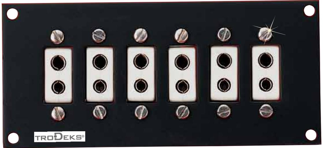
TRODEKS high-temperature jack panels feature ceramic connectors mounted in a steel plate for service temperatures up to 538°C (1000°F). These panels with UHX connectors are ideal when glazed ceramic or nylon connector panels would contaminate a vacuum system.
