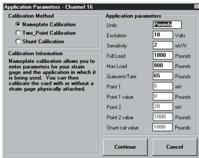
The OMB-DBK43A's software supports three calibration methods: nameplate, two-point and shunt
