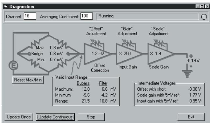
You can easily configure the OMB-DBK43A using its Windows software.
