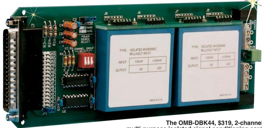
The OMB-DBK44, \$319, 2-channel multi-purpose isolated signal conditioning card
