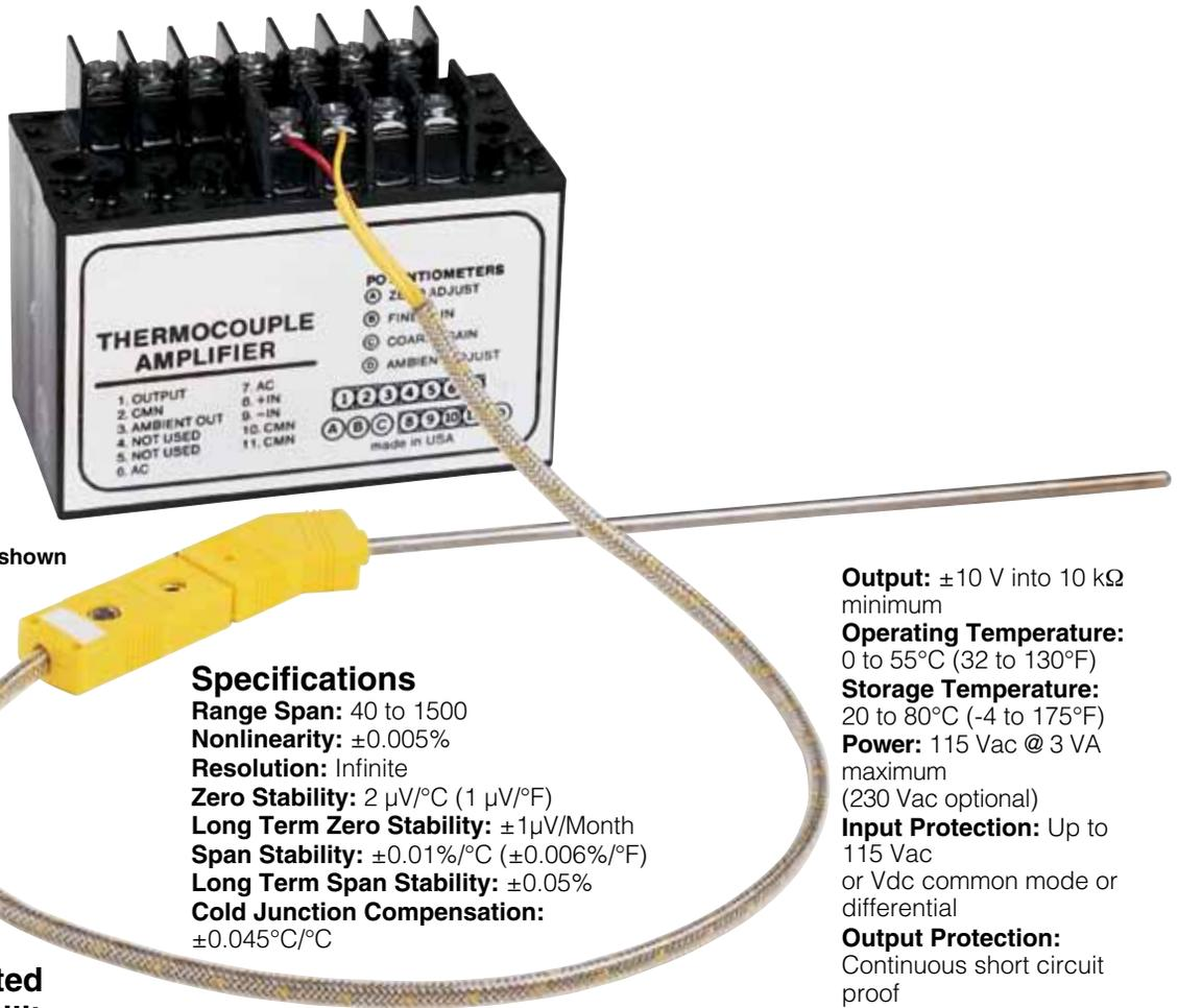
OMNI-AMP IV-13-115 shown with GKQSS-316G-12 thermocouple probe
