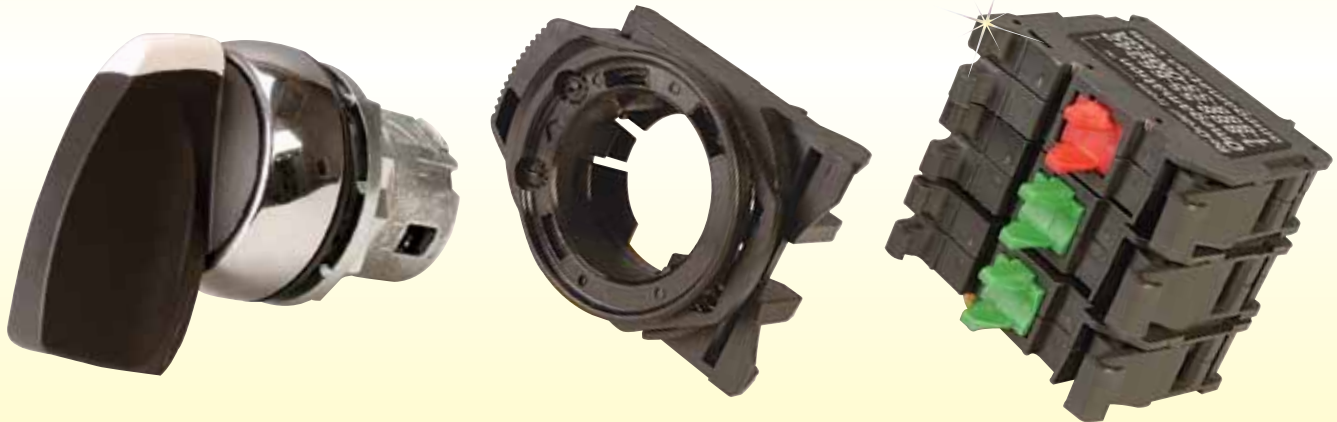
OMPBD7M-HM22PX01, two way metal selector switch with long knob. Each unit includes tool-less mounting latch and one normally closed contact block. Shown with two additional (up to 6 total per operator possible) normally open contact blocks, model OMPBD7-X10.
