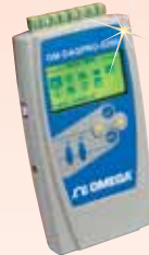
OM-DAQPRO-5300 handheld data logger.
